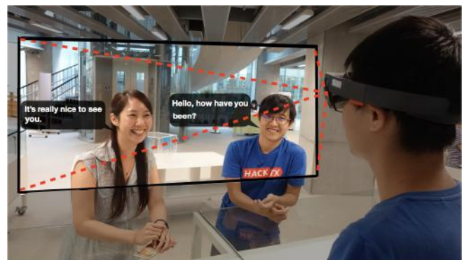
Figure 1. A proof-of-concept demonstration of SpeechBubbles. The user (right) equipped with a Microsoft HoloLens views speech bubbles adjacent to two speakers (left and middle).
