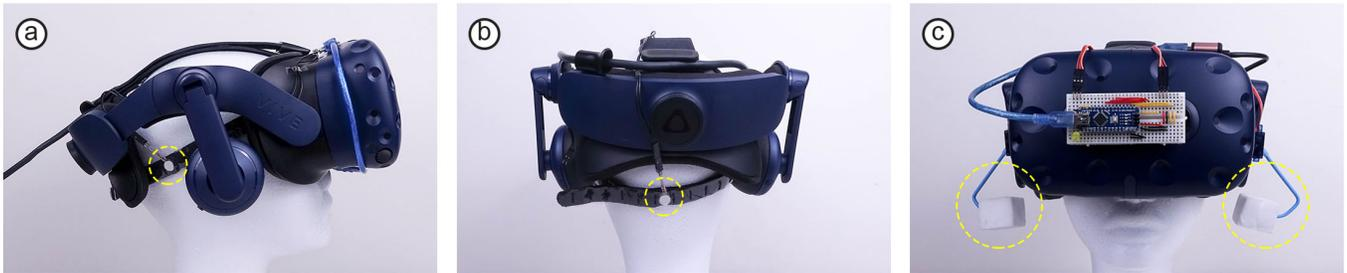
Figure 3. The setup for each category of tactile feedback: (a) 2-sided vibration, (b) backside vibration, (c) 2-sided tapping feedback replicated from PhantomLegs [37] project.
