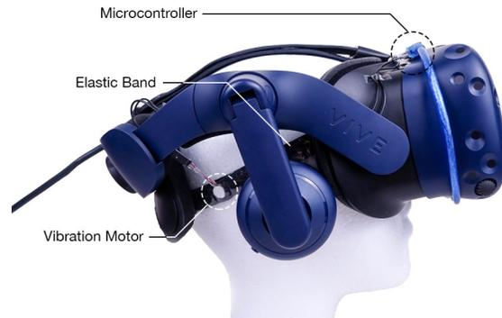
Figure 2. WalkingVibe prototype with 2-sided vibrotactile design.
