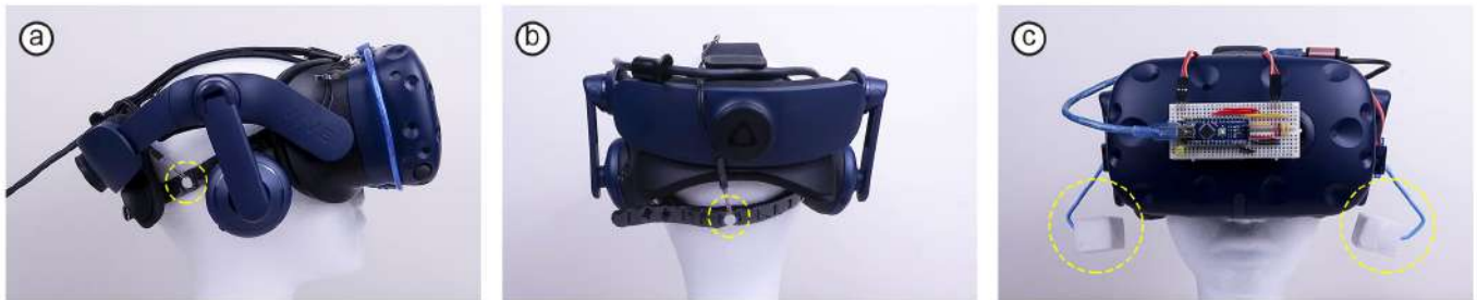
Figure 3. The setup for each category of tactile feedback: (a) 2-sided vibration, (b) backside vibration, (c) 2-sided tapping feedback replicated from PhantomLegs [42] project.
