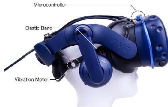
Figure 2. WalkingVibe prototype with 2-sided vibrotactile design.
