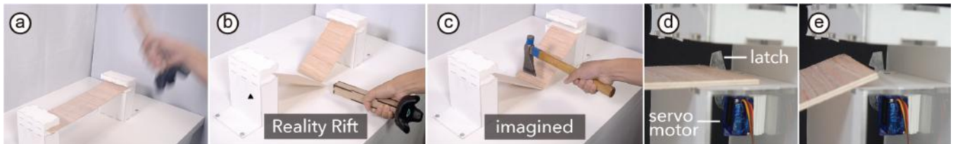
Figure 8: The platform releases the pre-cut wooden plate when the user strikes in the air with the generic stick, resulting in the imagination of using an axe.
