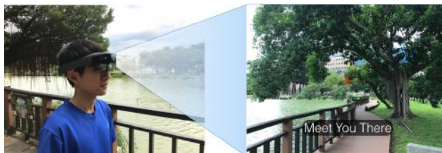
Figure 1: PeriText is a multiword reading interface for peripheral vision on Augmented Reality smart glasses. While (left) users focus on tasks in the real world such as walking, (right) PeriText provides real-time text information using rapid serial visual presentation, with words sequentially displayed below their center gaze, represented by the red crosshair.
