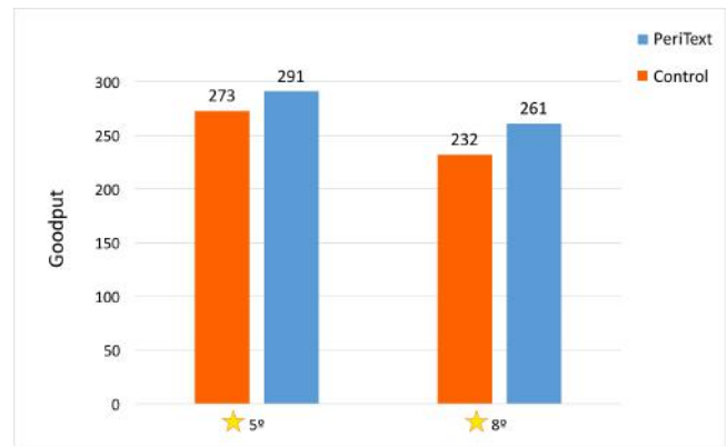
Figure 6: Goodput results of Study 2, comparing the performance of PeriText against control text. The goodput values are calculated as the average number of words perceived correctly per minute. PeriText resulted in 6.7% and 12.4% higher goodput values than control text, for both 5° and 8° eccentricities, and significance found through ANOVA.
